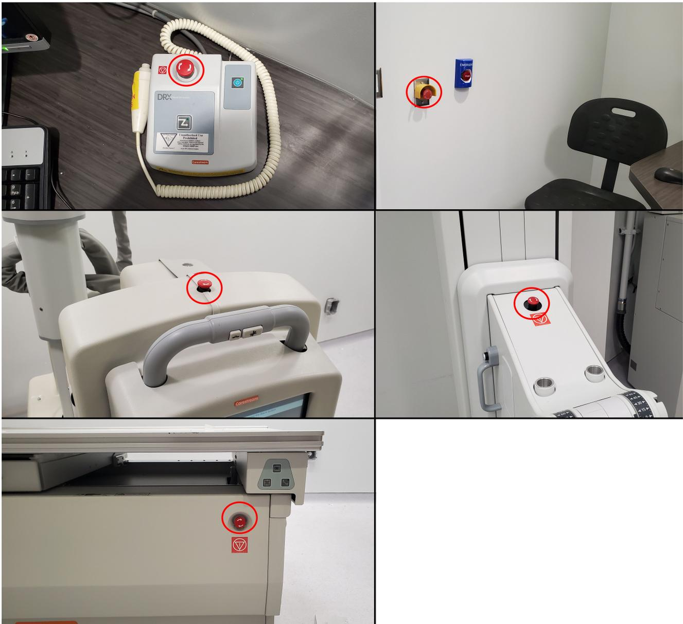
Figure 2: Emergency Stop buttons located on the gantry and on the operators' console.
